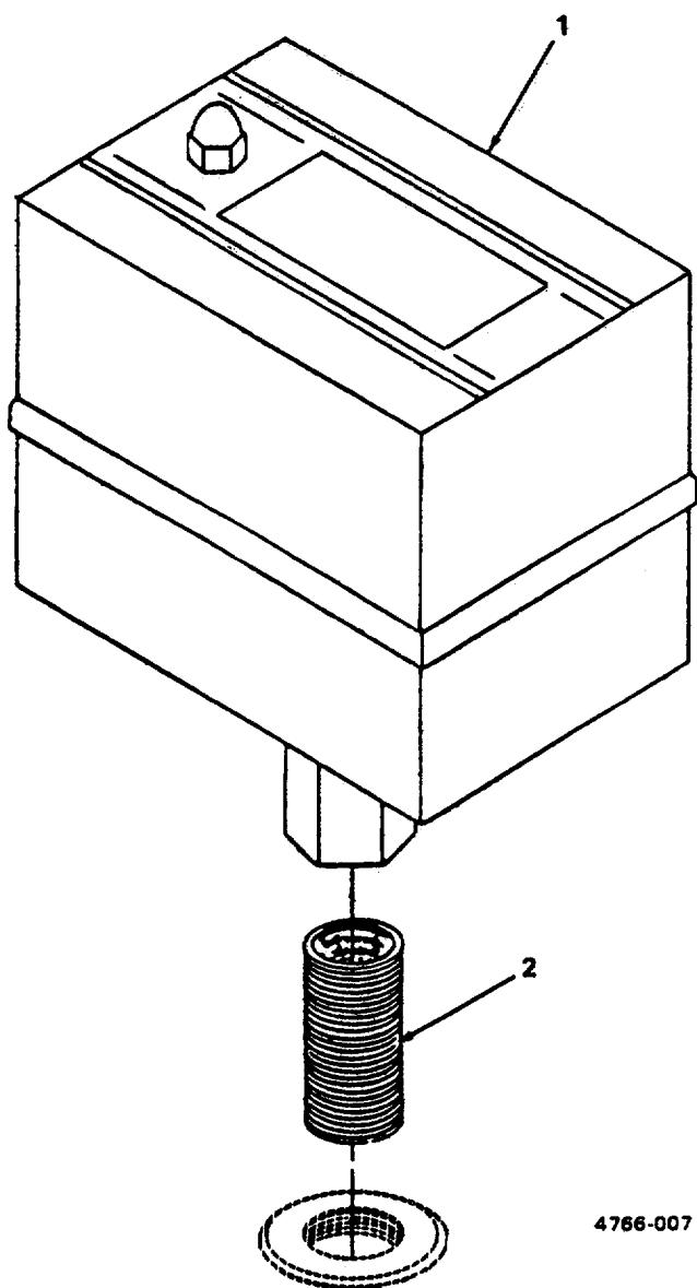
Figure 7. Pressure Switch.
